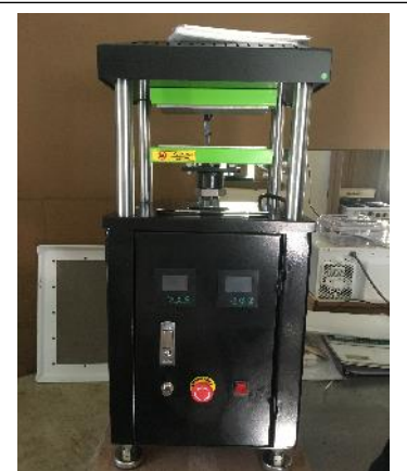
A rosin press consists of two heated plates which are intensely pressed together (typically between 300 to 600 psi used) to convert hashish into rosin.
